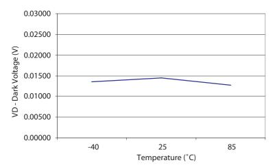
Figure 2. Dark Voltage vs Operating Temperature
