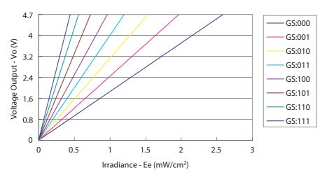
Figure 3. Voltage Output of Blue Channel vs Irradiance (lp = 460 nm)
