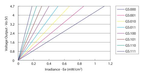
Figure 5. Voltage Output of Red Channel vs Irradiance (lp = 645 nm)
