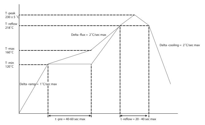
Figure 6. Recommended Reflow Soldering Profile
